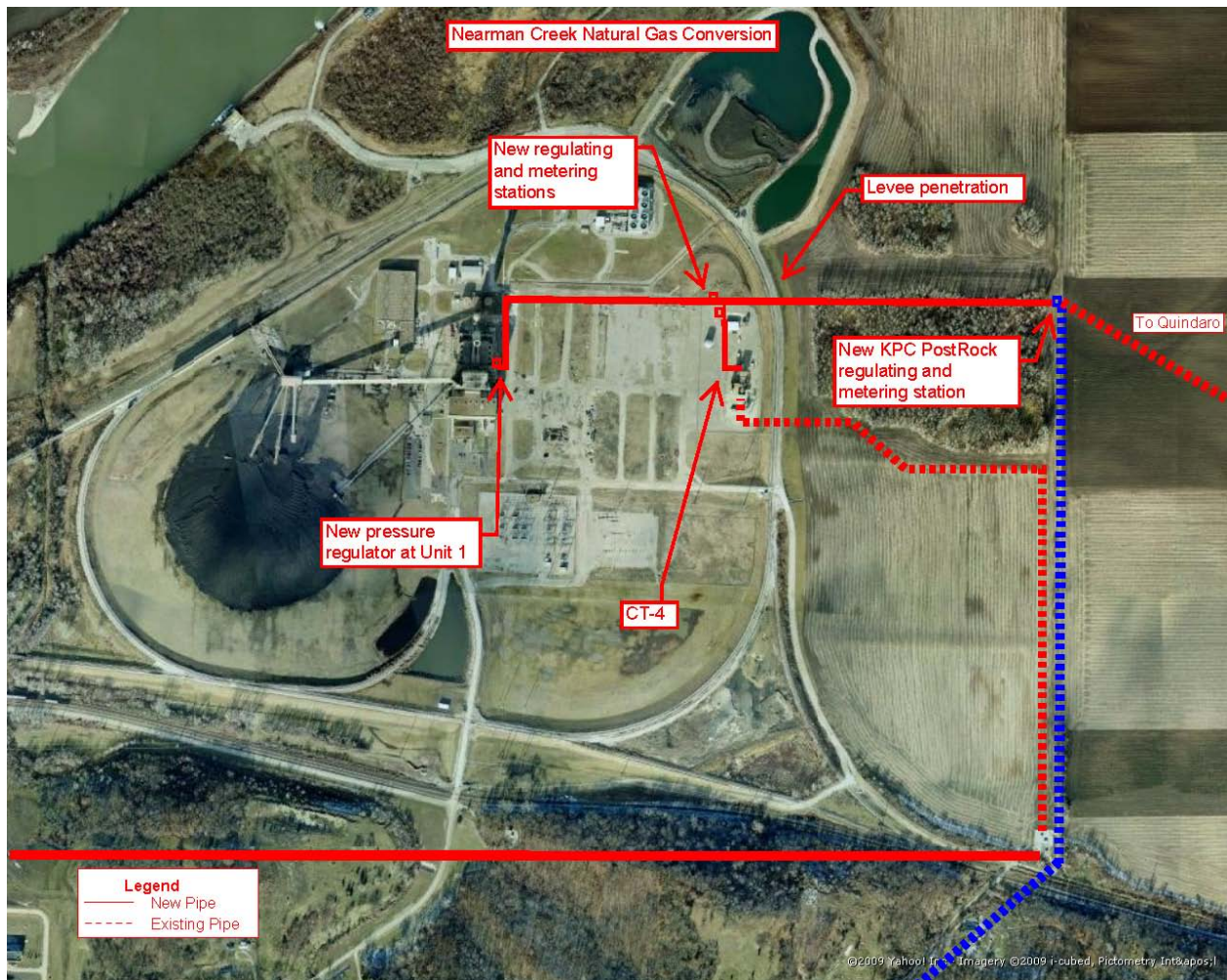
Figure 2-1 Gas Supply Pipeline Addition
